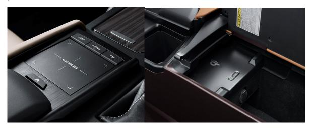
The ES also has the Remote Touch Interface with a smartphone-like feel and touchpad that is easy and intuitive to use. Vibration feedback on the touchpad helps driver awareness of cursor movements and button selection on the display.
