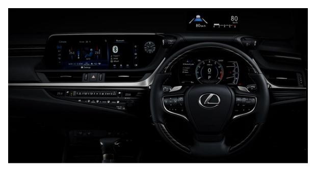
Drivers in the ES 250 Luxury can also refer to a Head-Up Display (HUD) that is the largest in its class with a display area of 260 mm x 97.5 mm. The high-resolution display is projected on the windscreen at an optimum visual distance so the driver's eyes can readily focus on objects in front of the car as well as the display. Information shown on the display are the road and engine speed, gear position, Dynamic Radar Cruise Control status and Land Tracing Assist warning.
