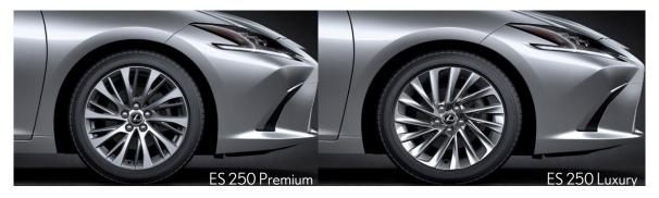
18-inch alloy rims are fitted on all variants, with the ES 250 Luxury wheels having Hyper Chrome Metallic Coating and a Medium Gray Metallic Coating for the ES 250 Premium. Similar to the LS wheels, the ES 250 Luxury comes with a noise-reducing hollow rim structure which helps reduce the resonance sound generated by the tyres. Tyres sizes are 235/45R18 for the ES 250 Luxury and ES 250 Premium having 215/55R18.
